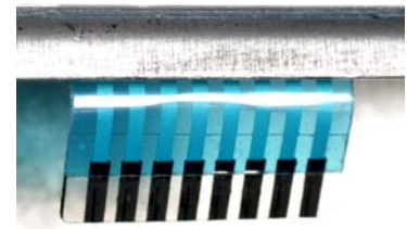
Figure 2: A bare ribbon cable extends from the new display assembly. This must be carefully inserted into the connector block on the display side of the board, which was removed from the failed display.
